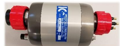
Stand-alone Motor Controller (SMC) Bottle w/o connectors \varnothing 4.72'' \times 5.86''
